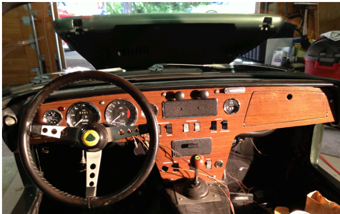
Dash with added voltmeter and oil pressure light. An MG radio blank is a perfect match for the ashtray.
